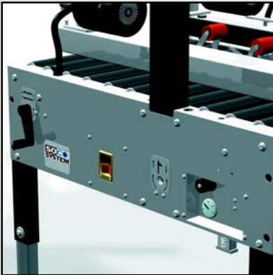
Crank Handle adjustment for carton size
