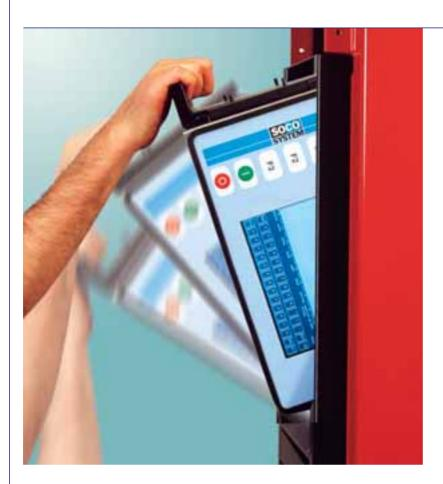
The palletising robot is controlled by an IPC-Controller, which is located in one of the pillars. When not in use, the IPC-Controller can be slid into the pillar – securing the electronics in the best possible way.
