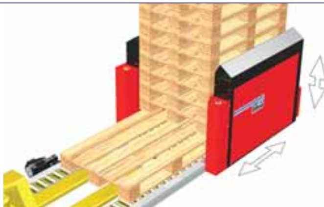
This Multi version stacks/destacks the pallets from pallet roller conveyors of heights as low as 90 mm. Here shown with 2-parted infeed/outfeed conveyor.
