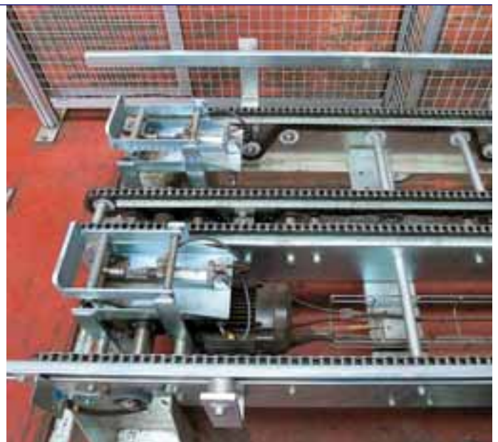
Chain conveyor system for \frac{1}{4} plastic pallets. The system is equipped with pneumatic stops for precise positioning of pallets at Dansk Kaffe Kompagni in Denmark.
