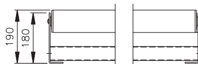
▲ Non-driven conveyor of height 190 mm.
