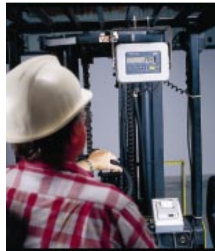
The WI-125 indicator linked with a WP-233 printer can provide an automatic hard copy of weight data.
