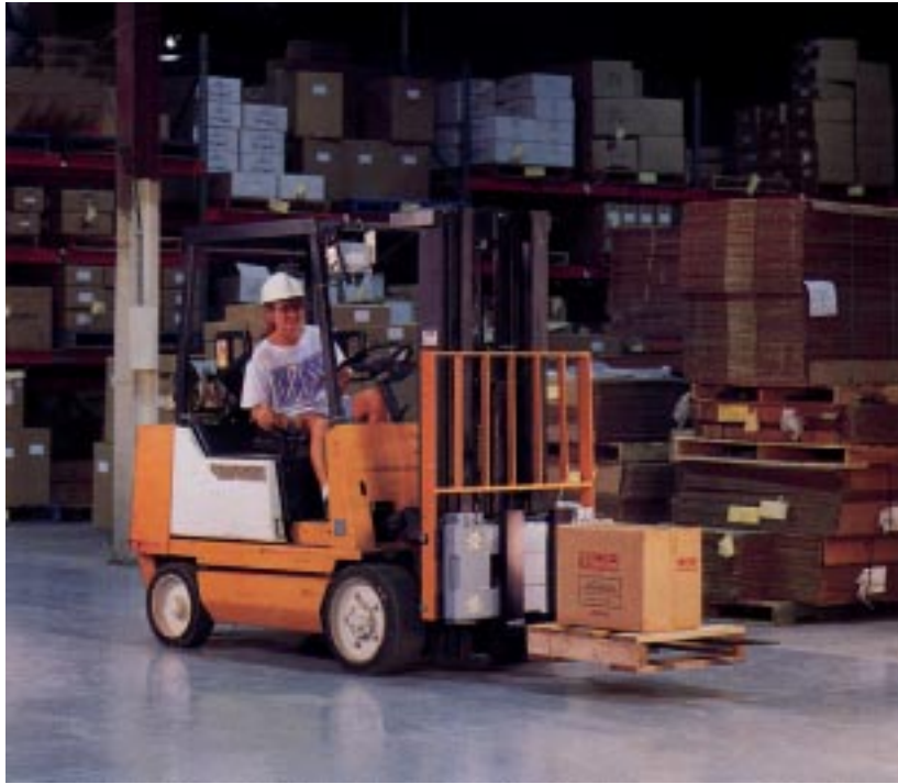
A combination of carriage assembly design, patent pending angle detection and a new Weigh Bar summing assembly allows the QTLTSC to weigh accurately with wide, normal or narrow forks.
