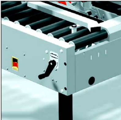
Crank Handle adjustment for carton size
